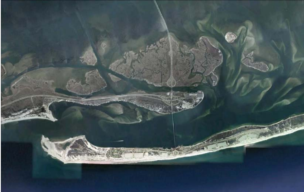
Figure 10. Aerial photograph of Fire Island inlet showing updrift offset beach and extensive flood shoal formation in the back barrier region.
