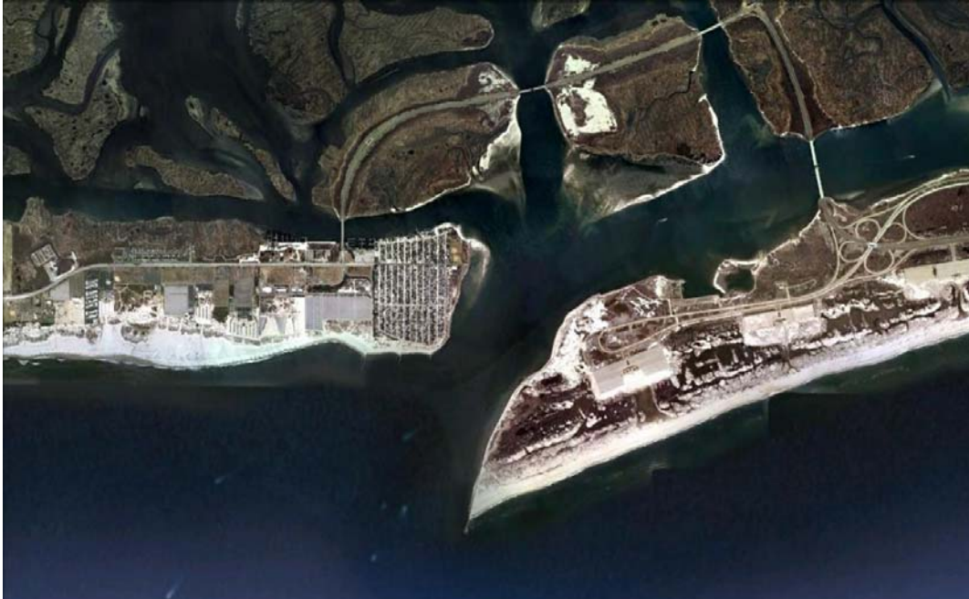
Figure 9. Aerial photograph of Jones inlet showing updrift offset beach and small flood shoals along the flanks of the back barrier marsh islands.
